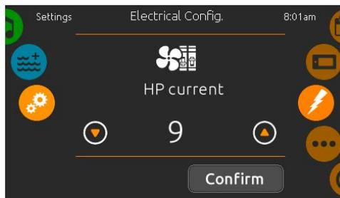
Please note that if there are two spa packs in the system (i.e. a SwimSpa installation), the master's unit's chosen unit configuration must support a slave unit. If after rebooting the chosen configuration does not support SwimSpa installations, the in.k1000+ will return (after approximately 45 seconds) to this configuration menu and prompt the user to select a configuration number again.
